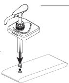
Pump connector is fully engaged when top surface of pouch fitment touches pump connector rim.
